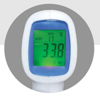
The backlight is green when the measurement temperature is normal
