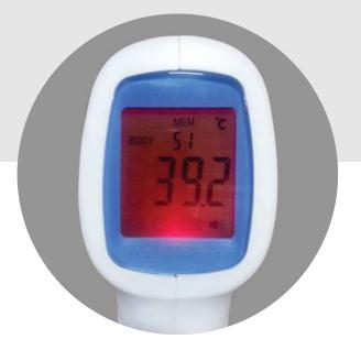
The backlight is red when the temperature setting is exceeded
